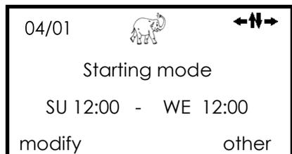
When this display is shown, the program will not start until it receives an **external signal** from, for example, a central control room or via a GSM telephone link. (requires suitable hardware)
