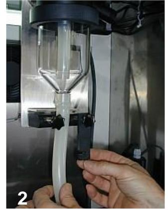
Remove the dosing hose either from the dosing glass or from the -X -Y distributor.
