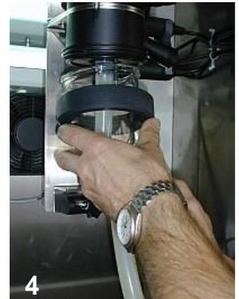
Clean the electrodes with a soft cloth and rinse the dosing vessel under the tap (figs. 7+8).
