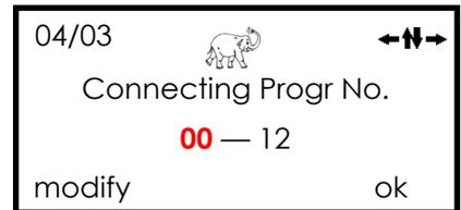
Here you can “connect” the used bottles to the bottles of a different program. (in this window to the bottles of program no. 03).
